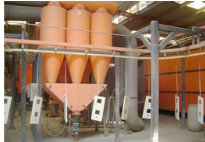
Conveyor belt for powder coating, (Source: Copyright by UNIDO)
